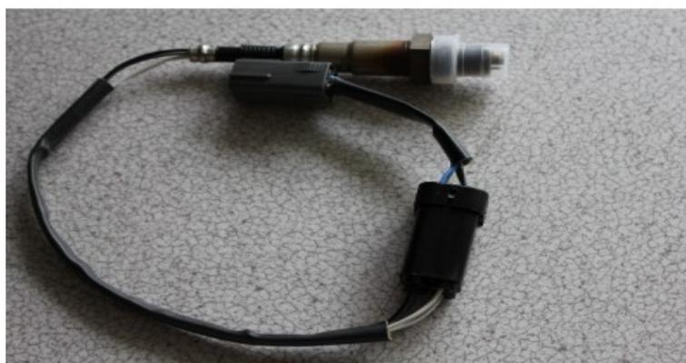
*VOICI AU SE TROUVE LE CONNECTEUR DE LA SONDÉ LAMBDA, IL EST JUSTE A COTE DU FILTRE A HUILE.*
